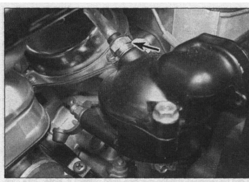
5.11 Temperature gauge sender unit location
