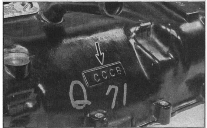
28.11 Main bearing bore diameter codes are stamped in upper crankcase half (arrow)
