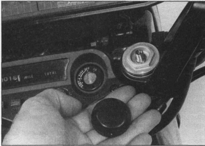
6.2 Remove fork bolt caps to reveal air valves on 700/750 models
