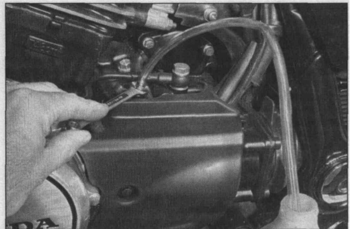
9.4 When bleeding the clutch connect tube to bleed valve as shown
