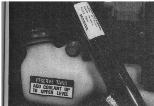
3.24 Reservoir tank mounting bolt on 1987 and 1988 700/750 Magnas
