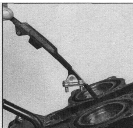
8.6 Rear camchain guide is bolted to crankcase
