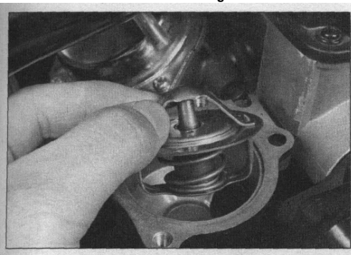
6.7 Lift the thermostat out of its housing
