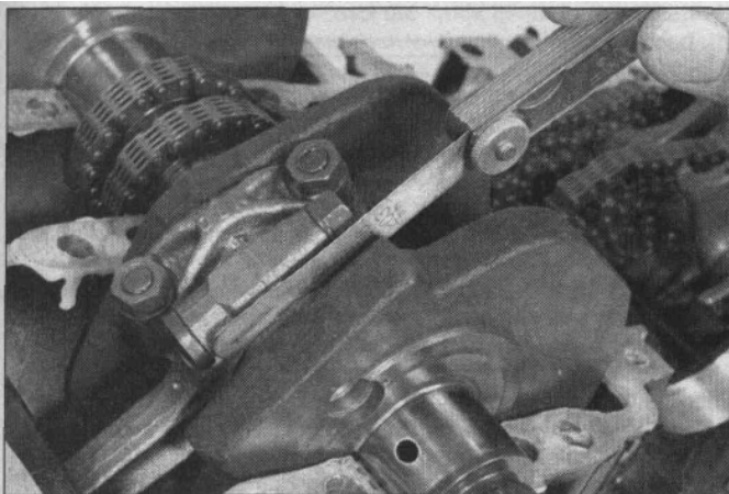
29.1 Measuring connecting rod side clearance
