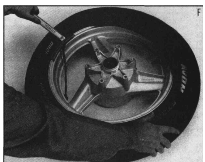
Use a tire lever to work the second bead over rim flange.
