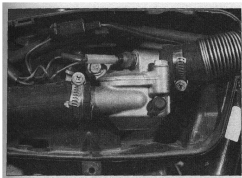
5.10 Thermostat is housed in right side air chamber on Magna models
