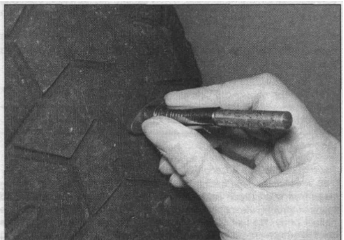
7.2 Measuring tire tread depth
