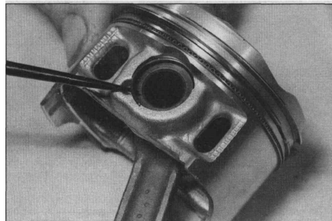
29.8 Pry out the circlip from the piston groove
