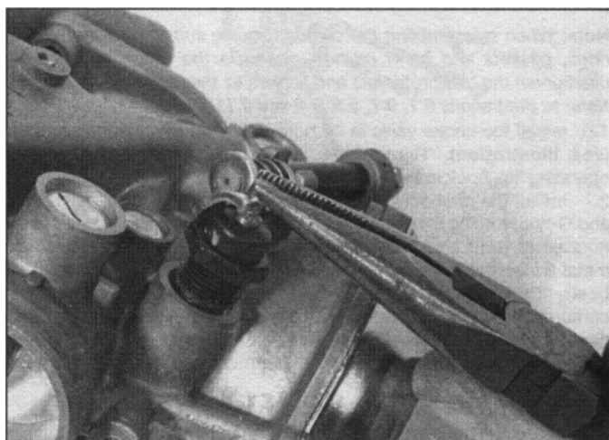
8.11 With the choke valve nut completely unscrewed, the choke valve can be pulled up and disengaged from its operating hook
