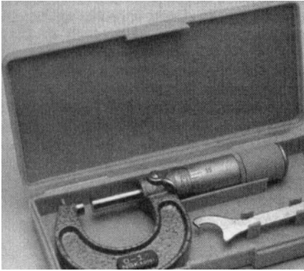
0-to 1-inch micrometer
