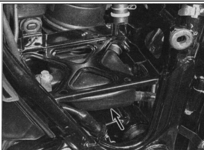
16.6 Crankcase breather separator tank (arrow) will be found in the mid-frame area - 700/750 Sabre location shown
