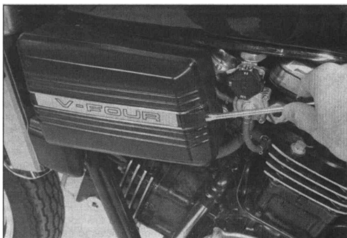
12.1 Pry out caps to reveal air filter cover screws on 1982 Sabre
