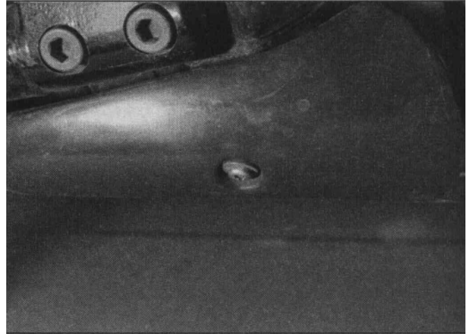
19.2c Rear section mounting screw
