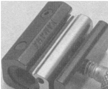
Spark plug gap adjusting tool
