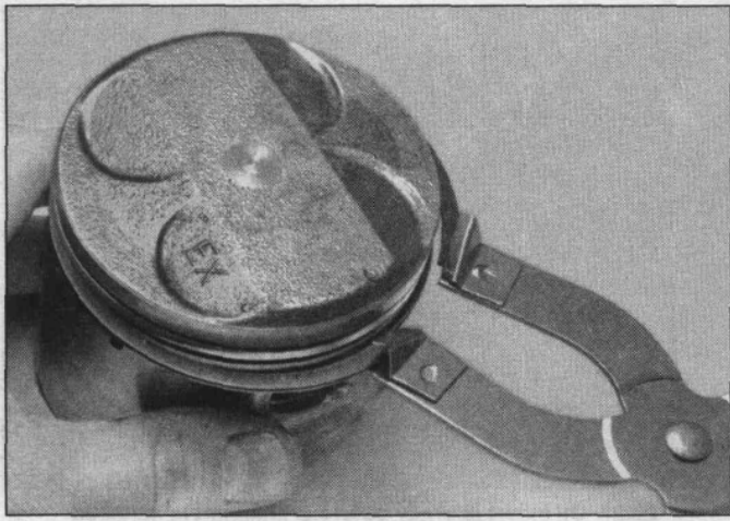
29.11 Use a ring removal and installation tool to remove top and second piston rings
