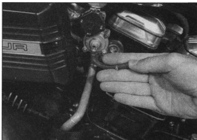
4.10 Checking the fuel valve diaphragm unit on 700/750 Sabres - suck on the vacuum hose then press your thumb tightly over the hose end
