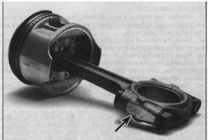
29.29 Connecting rod bearing bore size group and weight marking (arrow)
